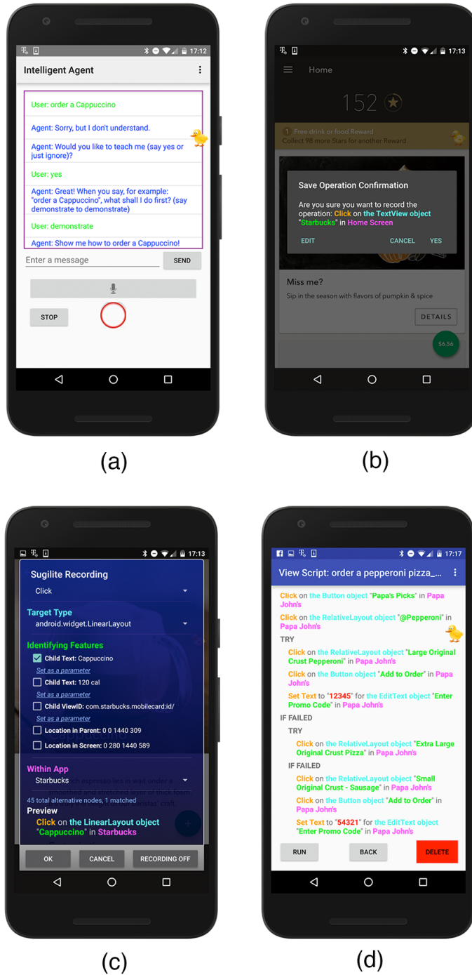
Fig. 1 Screenshots of the current version of SUGILITE prototype: (a) the conversational interface; (b) the recording confirmation popup; (c) the recording disambiguation/operation editing panel and (d) the viewing/editing script window (showing a different script).
